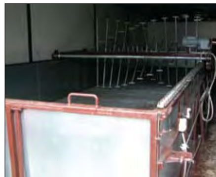
A "freezing box" used for blueberries at a handling facility in Kosovo.
